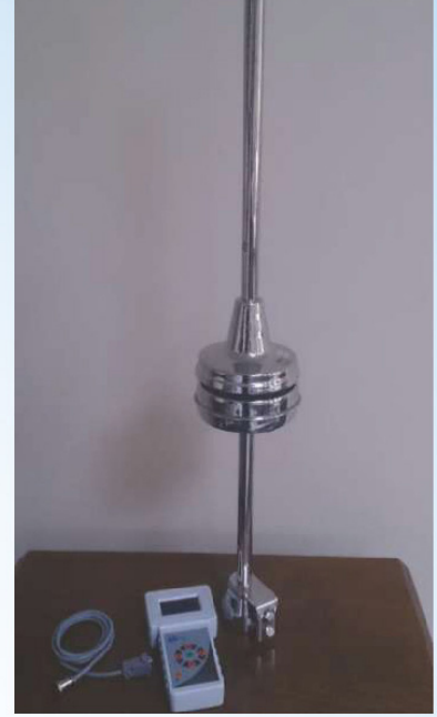
29 Paratoner test ekipmanları The Test Equipment of the Liva Lightning Rod with test cable
