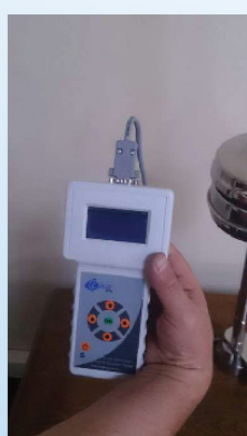
35 Test Kablosu Paratoner ve Paratoner Test Cihazı Soketlerine bağlandı The Test Cable connection was completed between Tester and Lightning Rod
