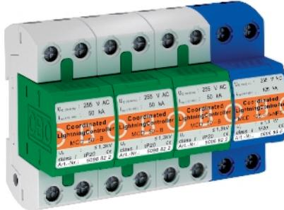
Combination arrestor, 4-pole, for use in TN-S and TT networks.
